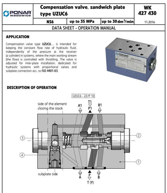
Main elements of the valve type **UZUC6**... are body (1), spool (2), spring (3) and logic valve (4) used to select higher control pressure from port **A** or **B**. For version UZUC6...**P**... (2-way version) the difference of pressures between port P and ports **A** or **B** acts on the spool (2), and after the initial spring (3) tension is overcome, the
