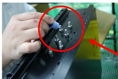
Fig. 5.15: Use non-magnetic tool to install the stator
